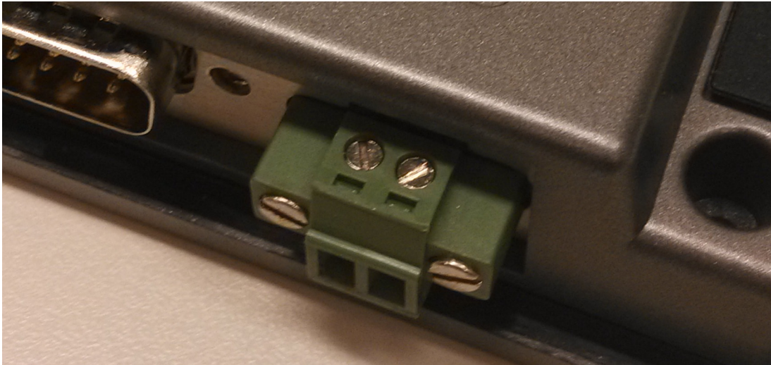
Figure 2.3 Power Line into the Power Receptor
